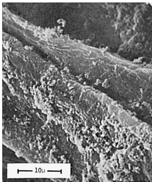
Fig. 7. Distribution of PSB 63/37 latex deposited at pH 6. A tendency to deposit as aggregates is apparent. At pH 3 the fibers are covered uniformly with individual particles.
